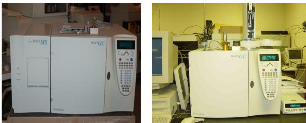
Figure 3. Gas Chromatography and Mass Spectrometry Devices.
