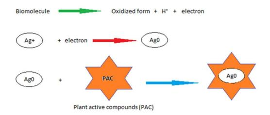
Scheme 1. The proposed mechanism for biosynthesis of AgNPs using plant extract.
